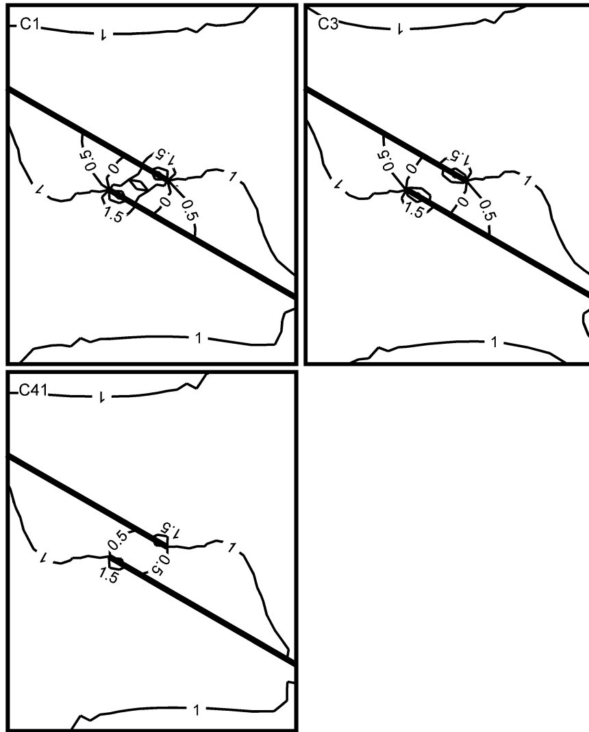
Fig. 9. Mean stress contour plots for selected C models of the extensional strike-slip fault bridge. Development stages of the bridge, fault friction and applied stresses are listed in Table 2. Mean stress values are normalised with respect to far field values as in Fig. 7. Contour interval is 0.5. Negative values are calculated in cases where \sigma_3 , and sometimes \sigma_2 , stress inside the bridge is negative.
