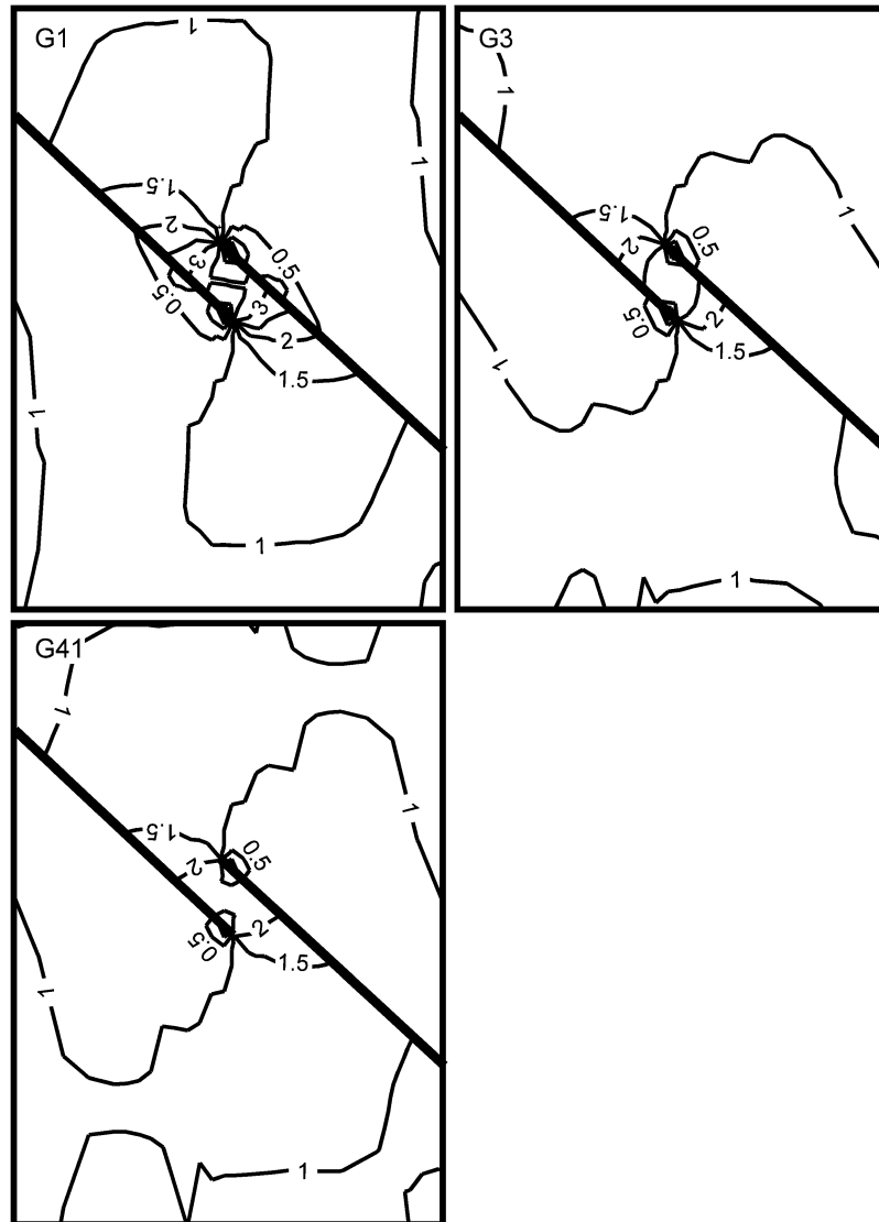
Fig. 7. Mean stress contour plots for selected G models of the compressive strike-slip fault bridge. Development stages of the bridge, fault friction and applied stresses are listed in Table 2. Mean stress values are normalised with respect to far-field values by division, where far-field values of the mean stress are 46.87, 28.67 and 25.63 MPa for stress magnitude ratio R = 0.1, 0.4 and 0.8 , respectively. Contour interval is 0.5.
